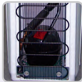
Hermetically sealed reciprocating compressor
